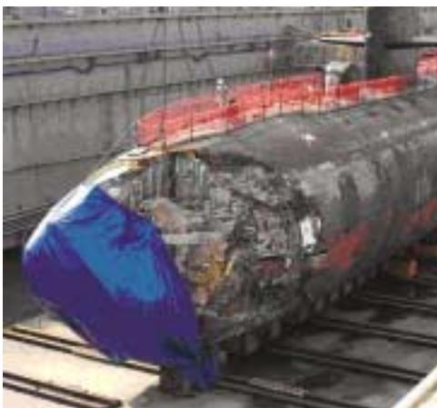
Photo showing the damage sustained to the *USS SAN FRANCISCO* (SSN 711). *USS SAN FRANCISCO* is the 24<sup>th</sup> submarine in the *LOS ANGELES* class and the sixth ship of that class built by Newport News Shipbuilding in Newport News, VA. She was commissioned on 24 April 1981.
